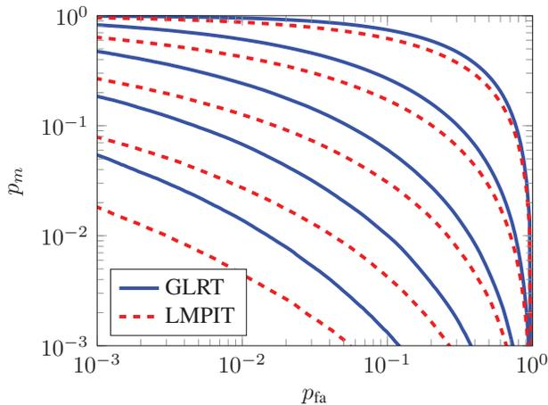
**Fig. 1.** ROC curves for different values of  $M$  in an experiment with  $L = 6$  antennas and  $\text{SNR} = 0$  dB.
